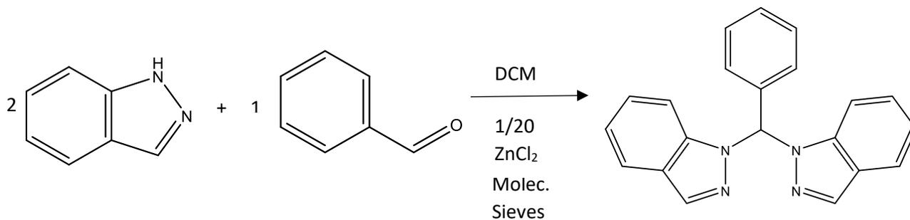
**Scheme 3:** Synthesis of **2**, indazole (left), benzaldehyde (center), diindazolyphenylmethane (right).
