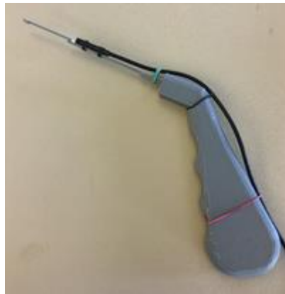
Figure 25: 3D printed model with scoop attachment and camera
