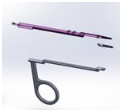
Figure 9: Exploded view of tweezer attachment
