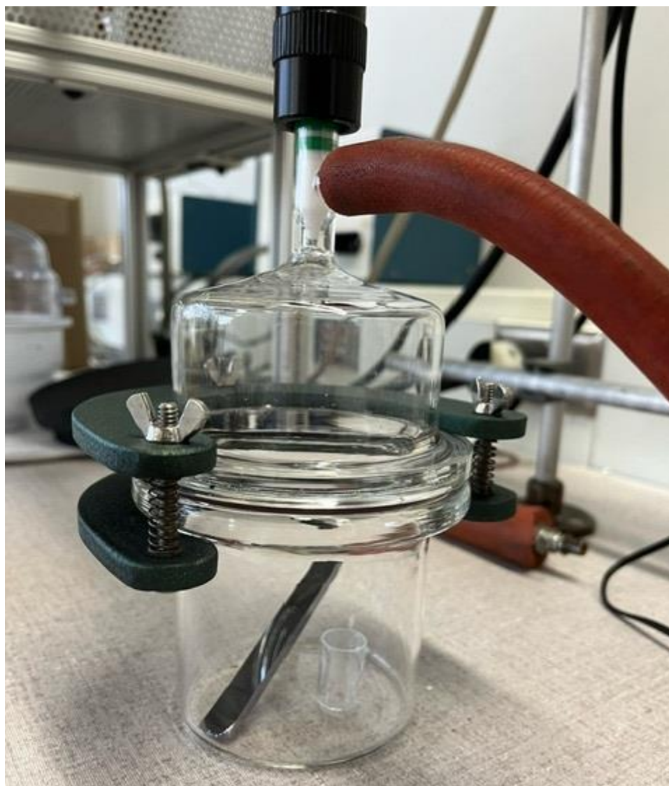
Figure 1. The experimental setup pictured above shows the process for placing the desiccator under vacuum. The silicon crystal is positioned alongside the initiator, which was placed in the small vial. The valve on top of the desiccator is open, and the orange tubing is connected to draw vacuum in the vessel. The green clamp ensures a tight seal between both glass pieces.
