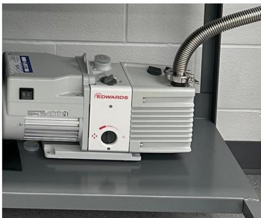
**Figure 11: Edwards RV12 Vacuum Pump on cart**
