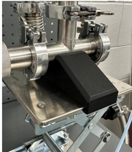
**Figure 15: Scissor stand to tube adapter**
