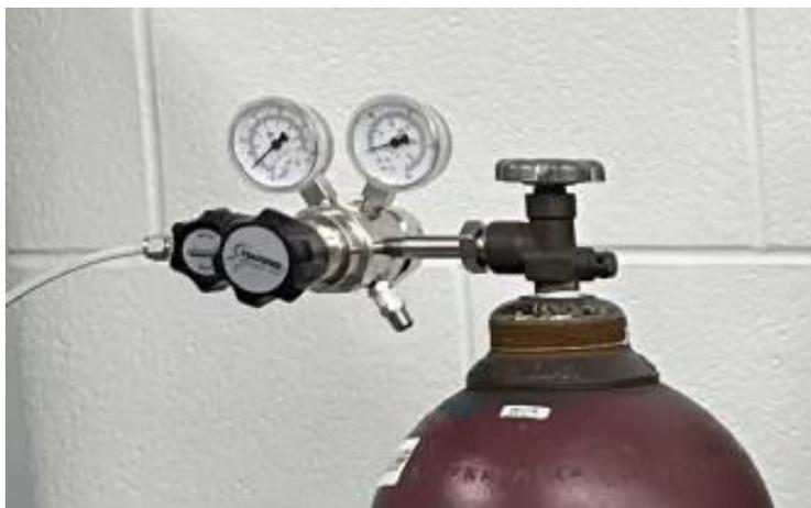
**Figure 25: Argon tank with regulator**
