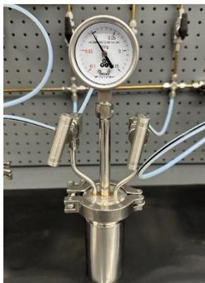
**Figure 6: Stainless-steel bubblers**
