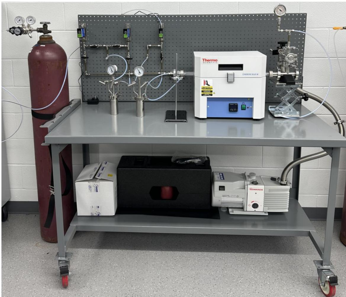
**Figure 16: Schaeffler iCVD reactor**
