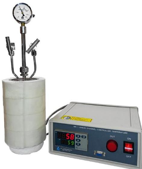
**Figure 7: Optional bubbler heating sleeve**
