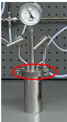
**Figure 27: Stainless-steel bubbler with opening highlighted**
