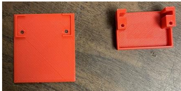
Figure 32 3D printed servo mounts
