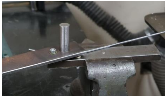
Figure 35 Nose gear bending
