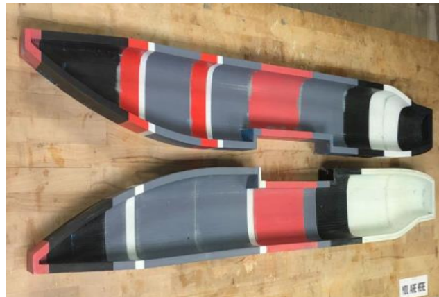
Figure 28 3D printed fuselage mold
