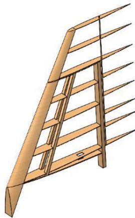
Figure 20 CAD model of the tail
