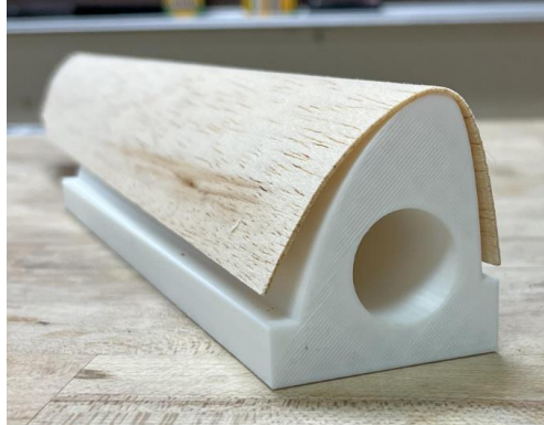
Figure 29 3D printed leading edge mold
