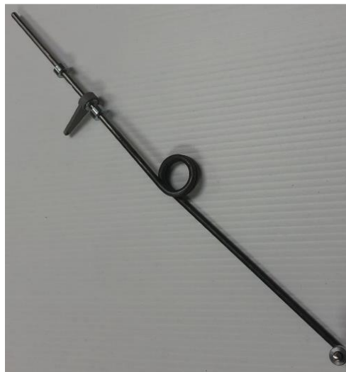
Figure 36 Bent nose gear
