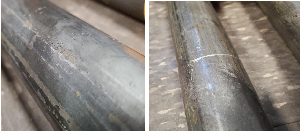
Figure 8: (A, left) Pre-straightening 150-gpm sample; (B, right) post-straightening 150-gpm sample.
