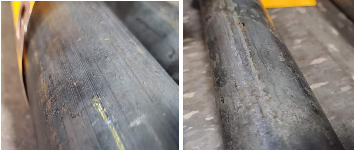
Figure 9: (A, left) Pre-straightening 400-gpm sample; (B, right) post-straightening 400-gpm sample.
