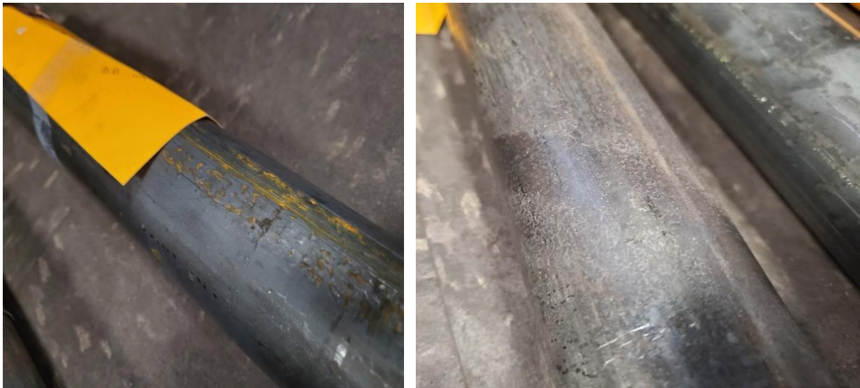
Figure 7: (A, left) Pre-straightening 0-gpm sample; (B, right) post-straightening 0-gpm sample.
