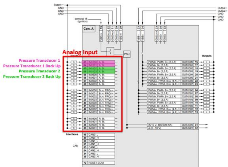
Figure 20: Analog inputs for the two pressure sensors in the PLC
