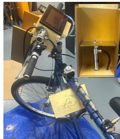
Figure 60: Pneumatics box placement on the back of the HMI box
