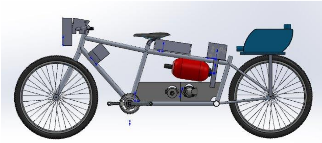
Figure 13: Left-side view of the bike assembly in SolidWorks, including the electronics boxes, pneumatic box, manifold, accumulator, pump and motor, reservoir, and
