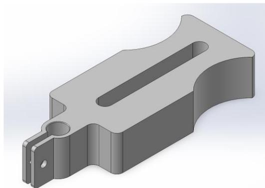
Figure 6 Borescope Mount
