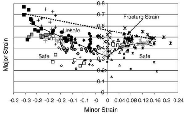
Figure 13 Typical Low Carbon Steel FLD
