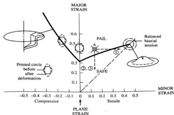
Figure 1 Forming Limit Diagram (Schey p. 409)
