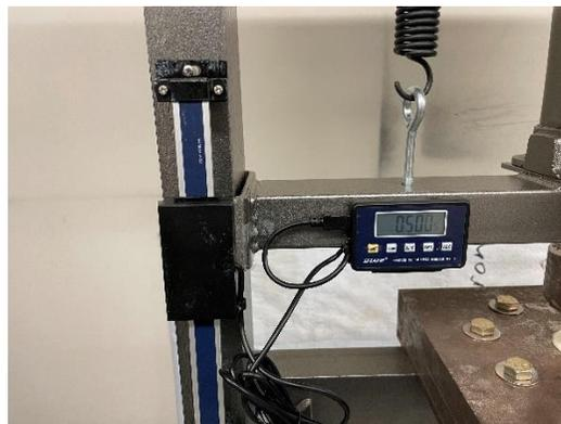
Figure 3 Digital Displacement Gauge
