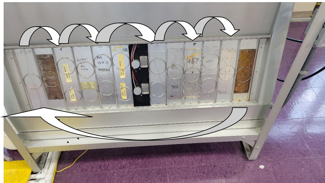
Figure 2: Schematic of the rotation pattern followed for QUV/spray chamber. Samples removed for data collection were taken from left to right, and sample holders without samples were filled with blanks.
