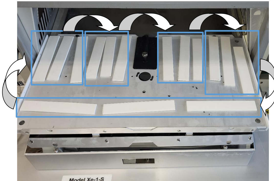
Figure 3: Schematic of rotation pattern followed for Q-SUN Xe-1 unit. Samples removed for data collection were taken from left to right. While this rotation schedule was followed for these sections of the testing tray, exact positioning of the samples was not monitored.
