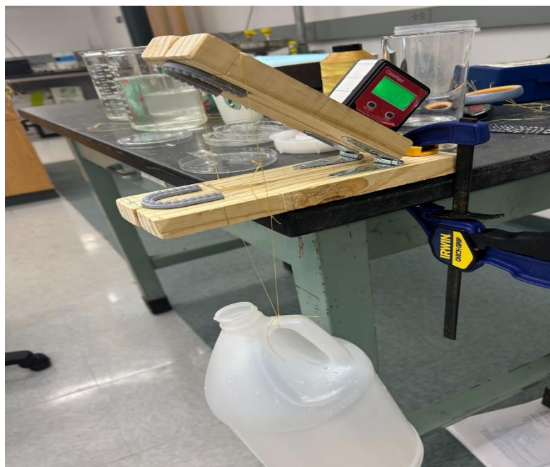
Figure 2. Bite simulator apparatus. Photograph of apparatus used for testing bite force of jaws at both standard position and offset alignments.
