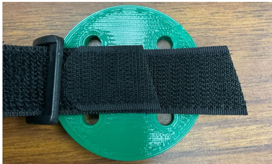
Figure 34: The modified hook-and-loop strap.
