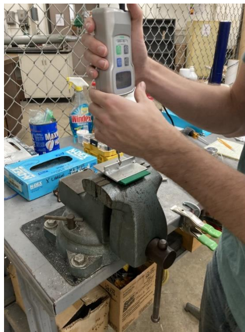
Figure 37: The PLA, gecko tape and aluminum testing part setup.
