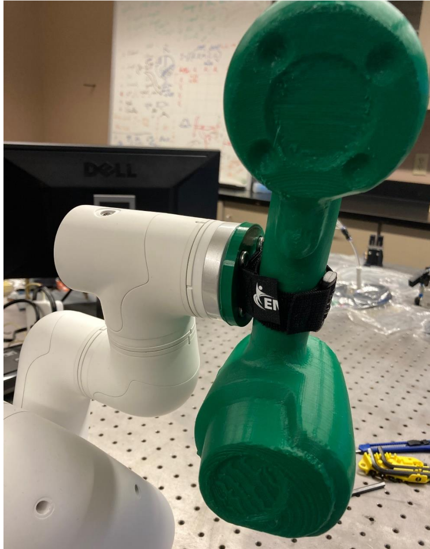
Figure 36: When the robotic arm is in the upright position, the forces acting on the gripper cause the printed 3D scanner to be held slightly tilted.
