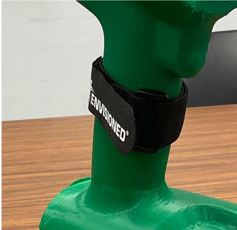
Figure 33: The initial hook-and-loop strap was unable to fully clasp due to the length of the strap being too long.
