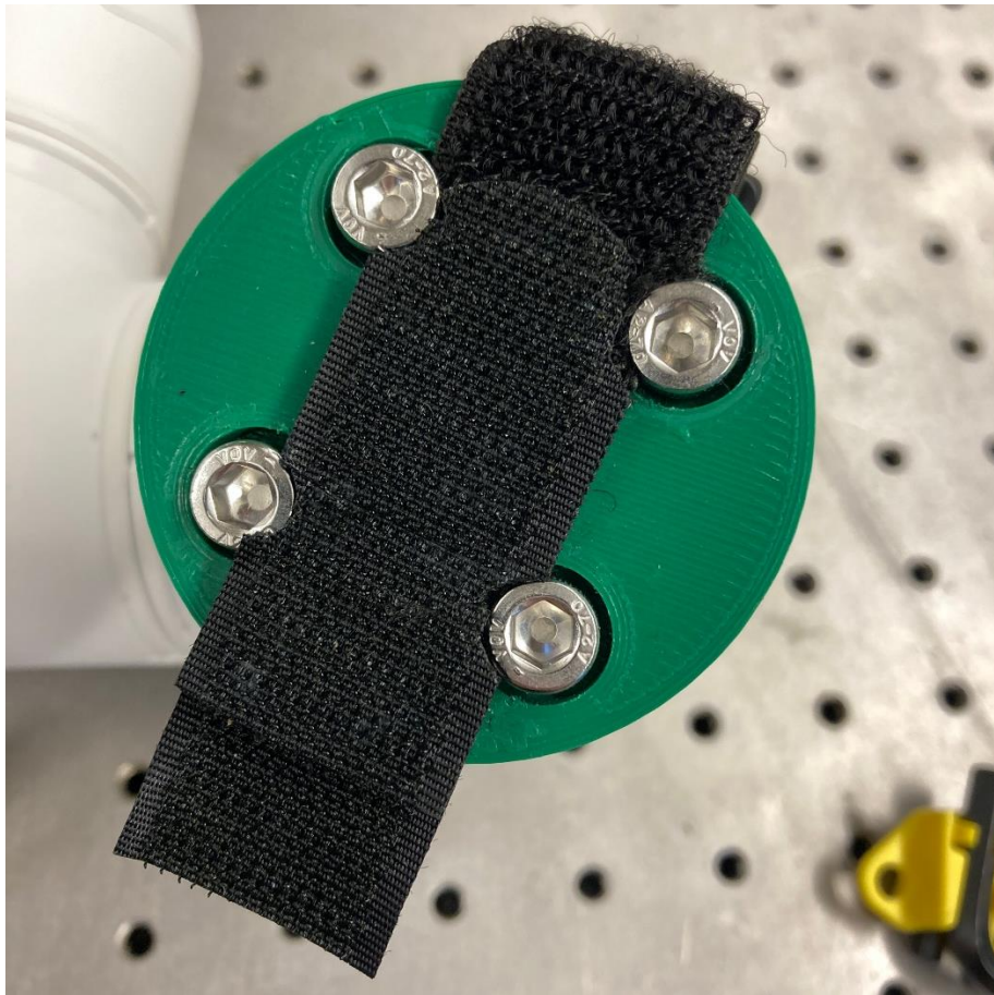
Figure 35: The final gripper attached to the end effector of the robotic arm. The area of the strap that interfered with the bolts was removed.
