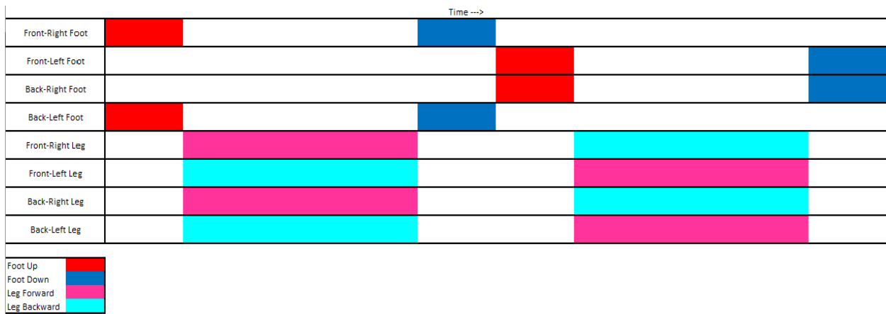
Figure 20: Gait diagram for the mobile robot.
