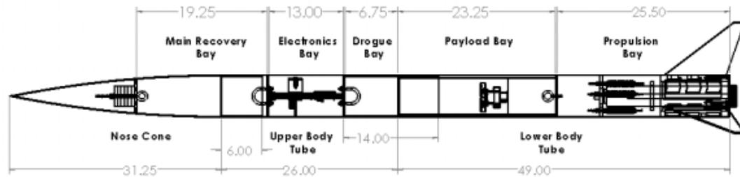
Figure 1: Example Rocket Layout
