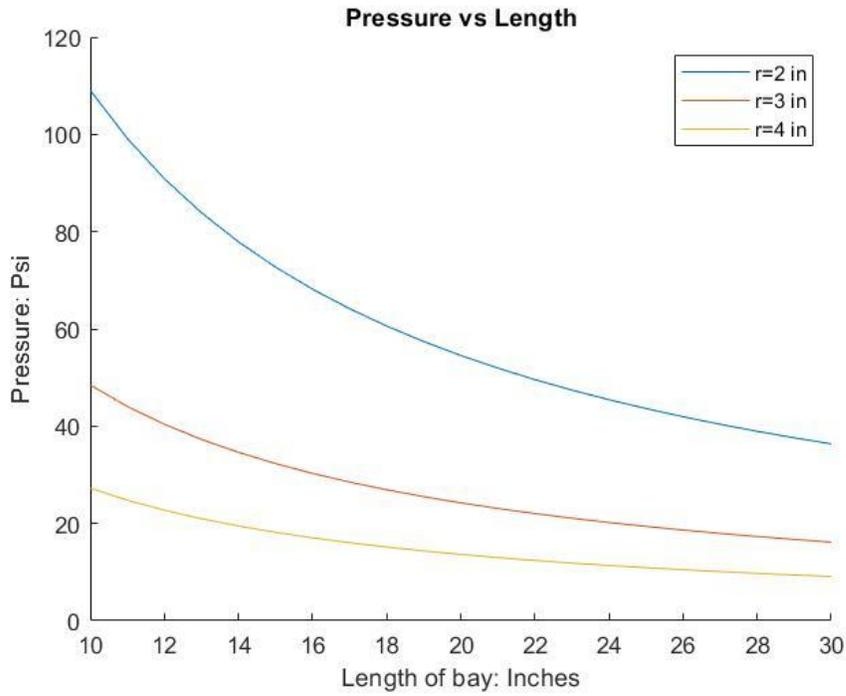
Figure 13: Display of Effects Radius has on Pressure for 30 grams CO2
