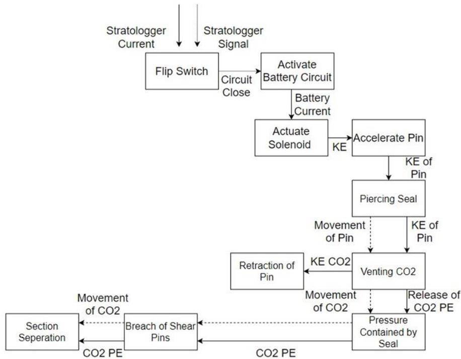
Figure 6: Function Diagram
