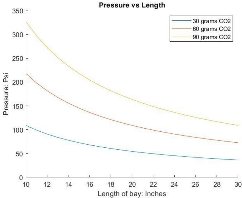
Figure 16: Display of Effects Different Cannister Sizes have on Pressure
