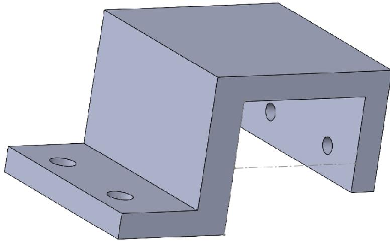
Figure 10: Connection to bulkhead
