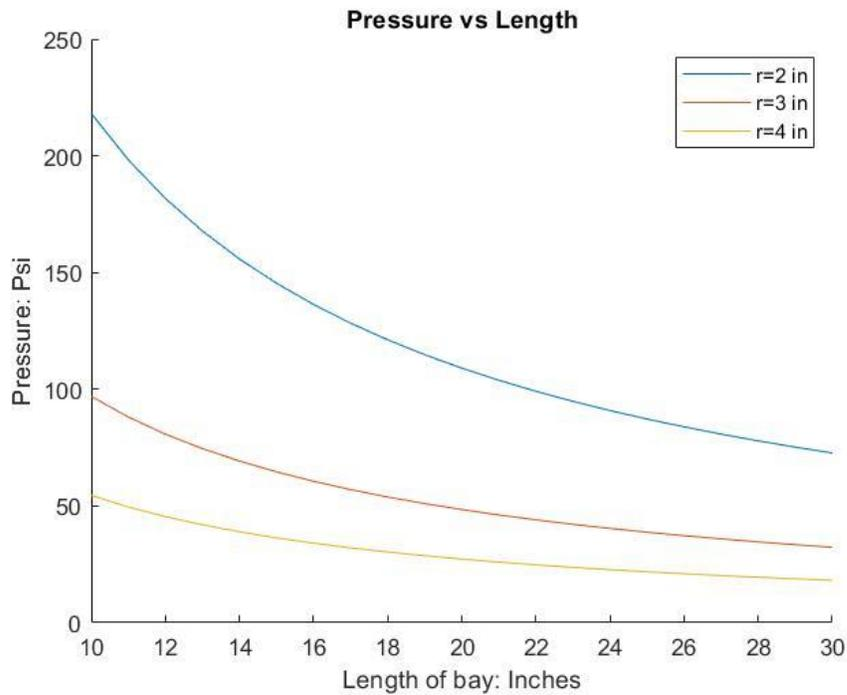
Figure 15: Display of Effects Radius has on Pressure for 90 grams CO<sub>2</sub>
