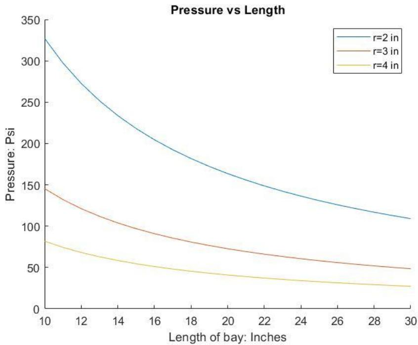
Figure 14: Display of Effects Radius has on Pressure for 60 grams CO2
