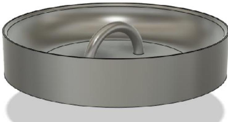
Figure 11: Shock Cord Connection Through Plug
