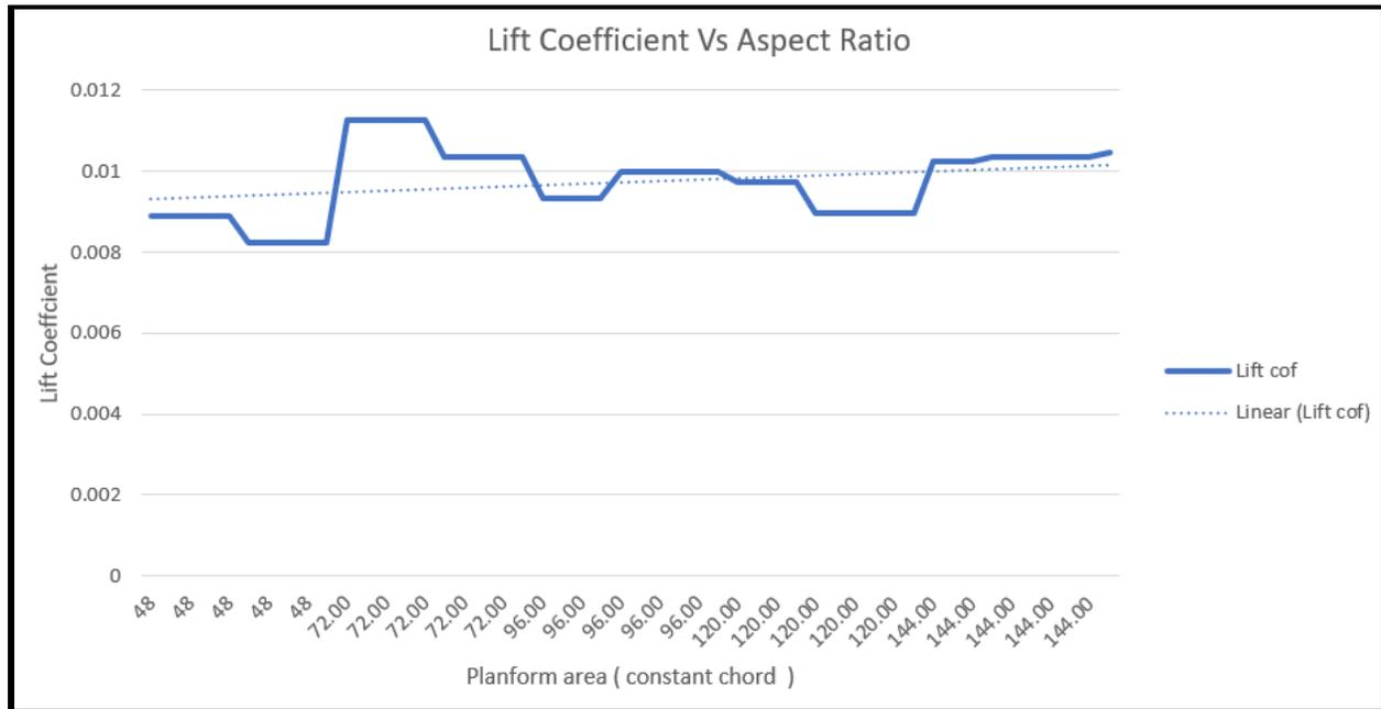
The above figure shows the lift coefficient vs aspect ratio. The coefficient value increases with aspect ratio at a constant chord. This is expected and adds some reliability to the results. Again there are the same errors as described in the drag coefficient graph.
