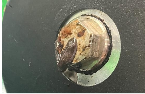
Figure 8: Contamination in Extrusion Process Resulting in Melting of Plastic
