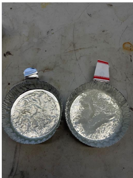
Figure 3. Pictured are 2 PPGDA-PEHA (1:2) mixtures, one with KCl added(right) and one without(left). Wrinkling of the structures provides insight that ample crosslinking did occur.
