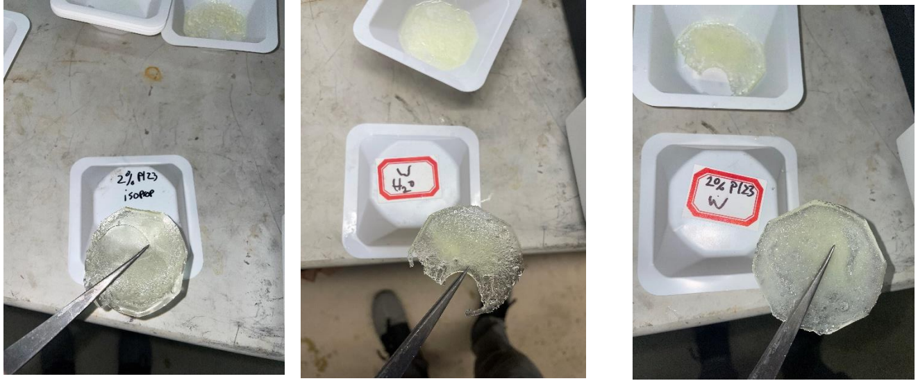
Figure 8 Solutions of PPGDA mixed with different solvents to create a porous structure
