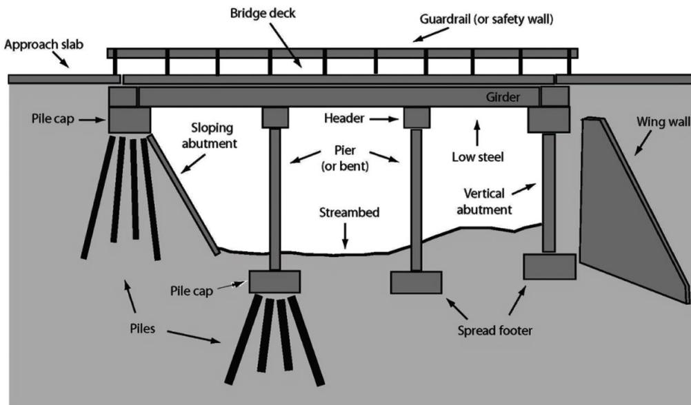
Figure 1: Substructure Diagram
