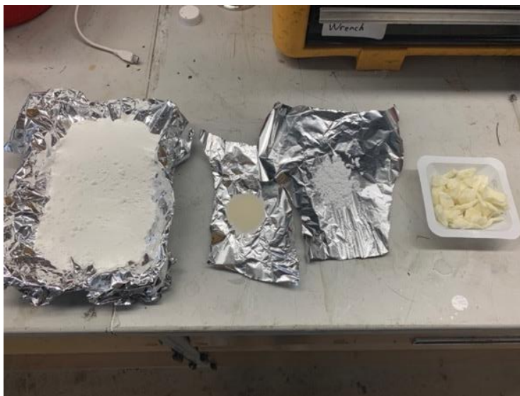
Figure 1: Array of general appearance of the sorbents tested, with TPSENa on the left, ASPEN in the middle, and PU on the right.
