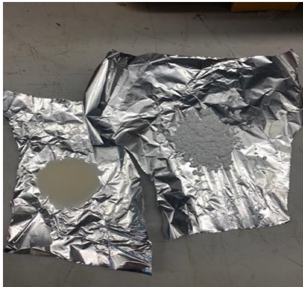
Figure 6: Visual of powder (left) and chunk (right) ASPEN sorbents
