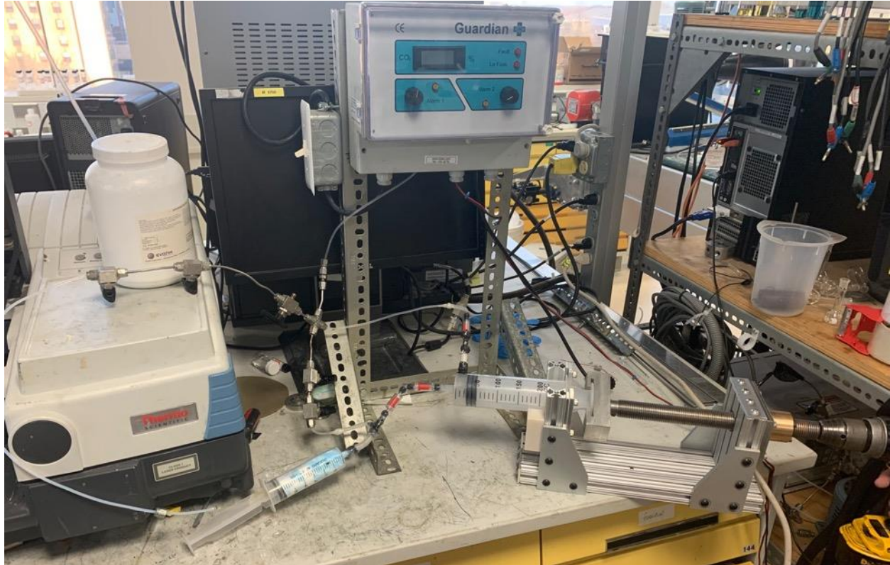
Figure 10: Visual of the CO 2 analyzer with the vacuum swing attached.
