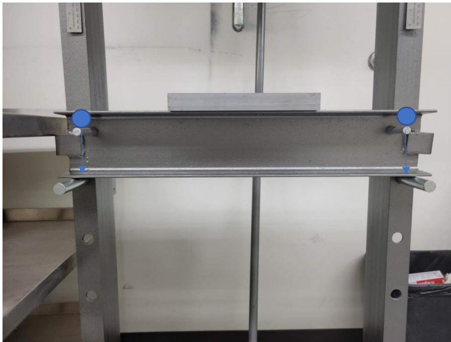
Figure 8: The upper position pin holes exist behind the apron in this image, focusing on those move them downward 1.5 inches to support the new height to set the pins to allow testing and assembly at
