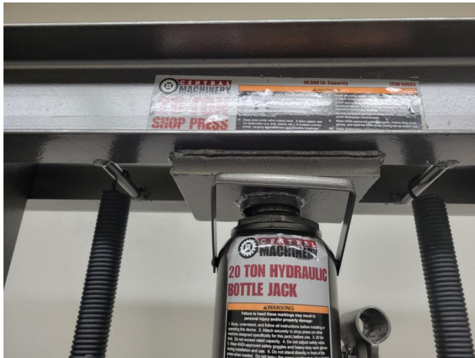
Figure 4: Cylinder misalignment for centering on upper assembly
