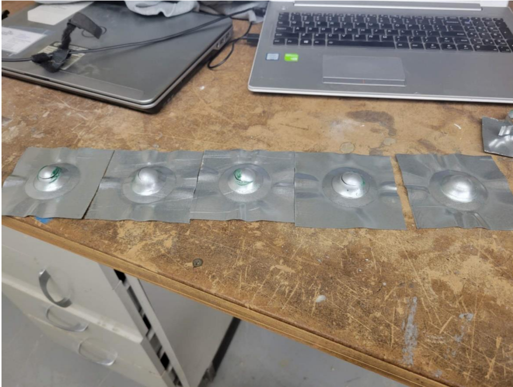
Figure 12: Initial Tests of 4-inch x 4-inch samples with varying wrinkling in each due to inconsistent tightening of bolts caused by incorrect and improper calculations
