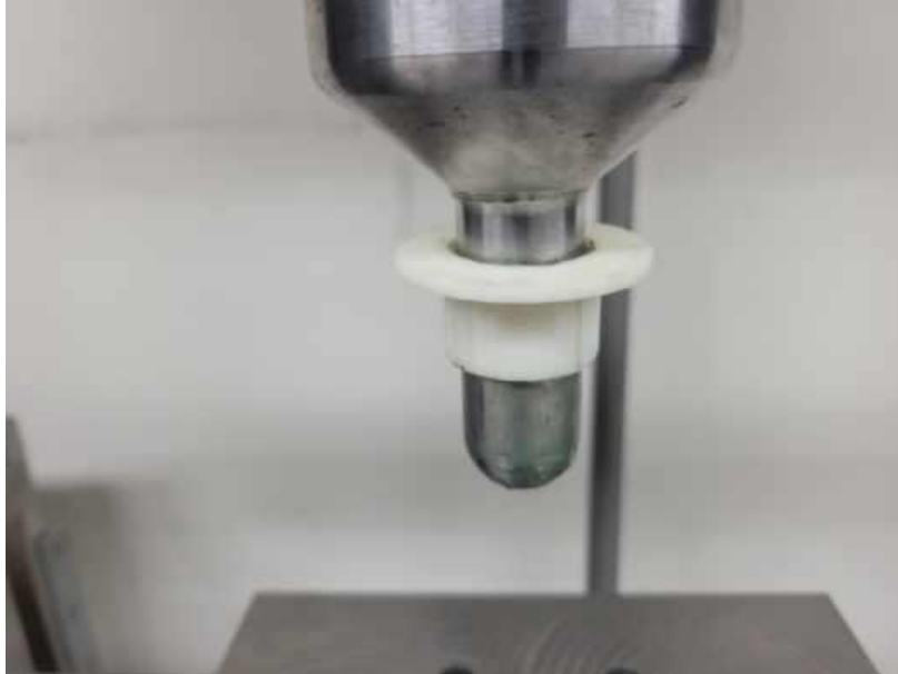
Figure 7: 3D Printed ABS shim shown with tight tolerancing to the punch
