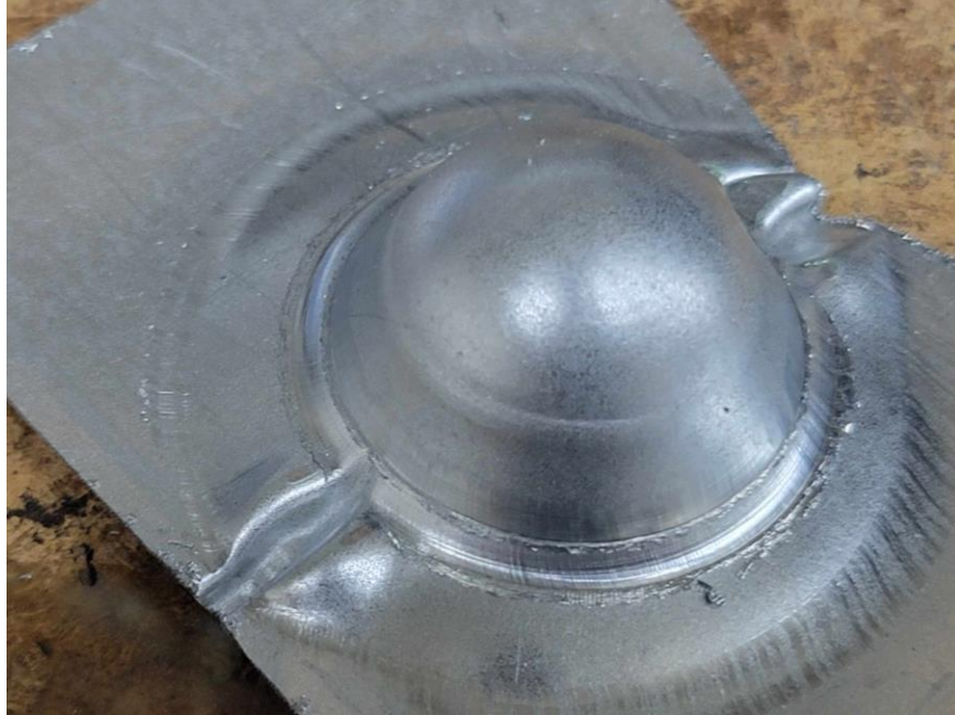
Figure 14: Initial Testing of 4-inch x 2.5-inch sample showing problems with wrinkling caused by incorrect holding force as well as interference on lower die chamfer which should be fileted instead to get rid of the sharp edges that the material catches itself on and improve metal flow [6]
