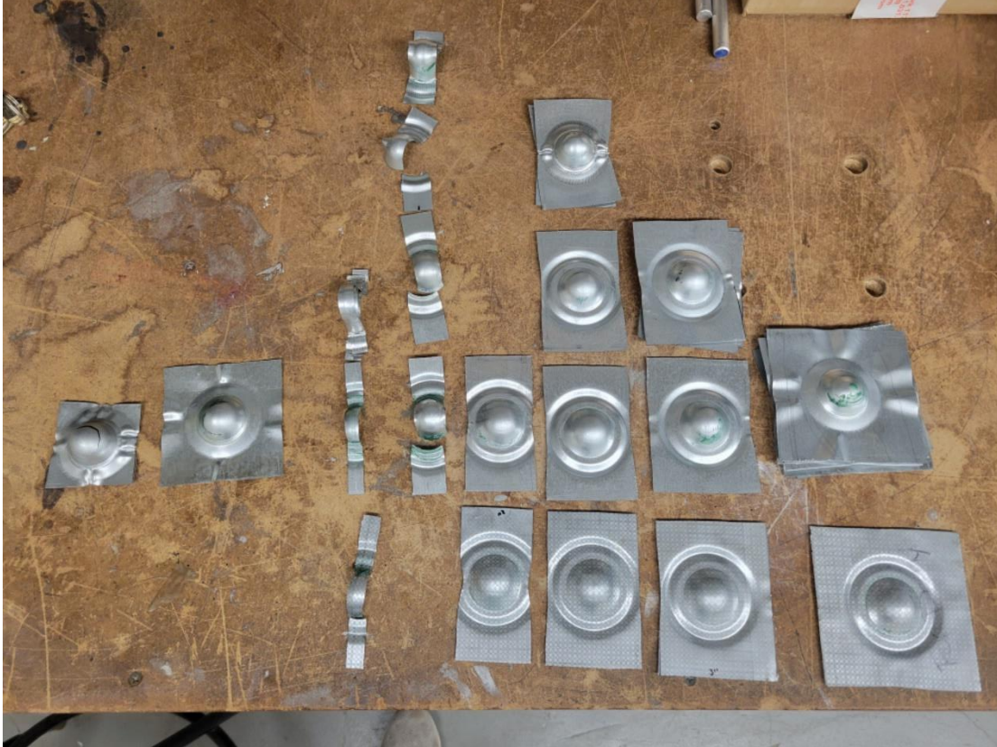
Appendix F10: All Samples that were tested and circle grid etched blanks in bottom row
