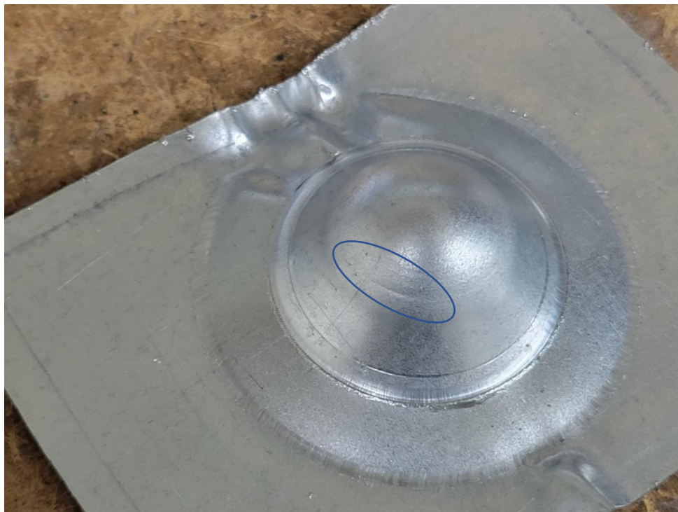
Appendix F11: Example of necking point (Stretched strip of material circled)
