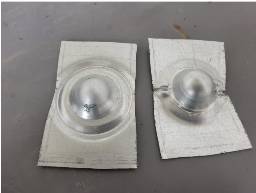
Figure 15: Improvement of blank holding force in testing from the initial calculations provided on the right to the corrected torque on bolts on the left
