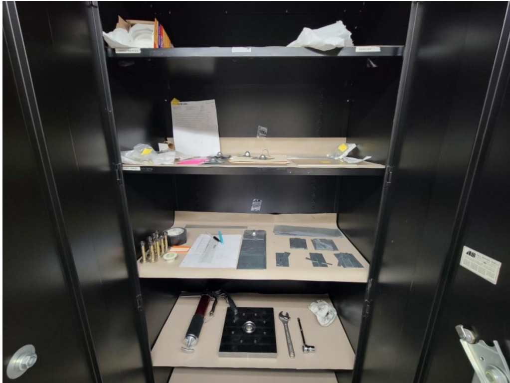
Appendix F6: Cabinet Located next to stand contains, dies, grease, wrenches, bolts, nuts, washers, 3D printed puck and shims, D2 Dies, and material for testing. Everything Necessary for the Dome Testing Stand.
