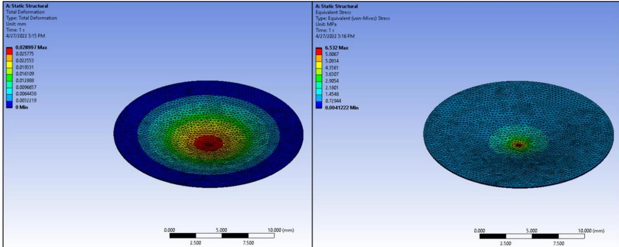
Figure 10. Ansys Workbench to calculate Total Deformation (left) and Equivalent Stress (right)
