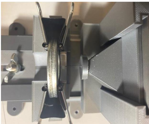
Figure 9. Example of Electrode Substitute Insertion
