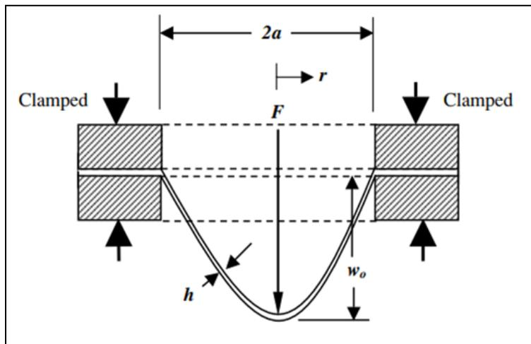
Figure 11. Sketch of a Circular Membrane Deformed by a Central Point Load
