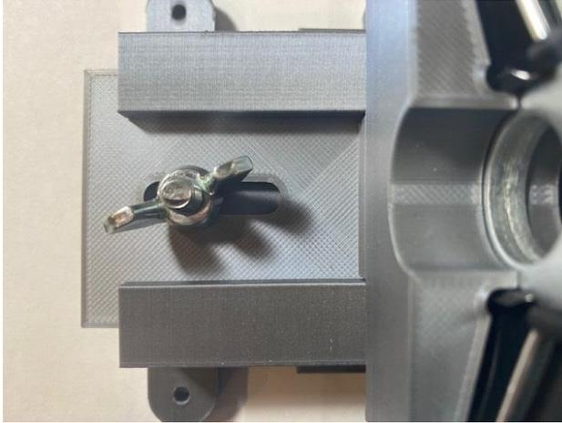
Figure 8. Adjustment Capabilities for Cochlear Implant Training Model Prototype
