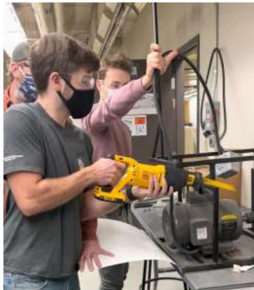
Figure 22: Team cutting the frame using a reciprocating saw
