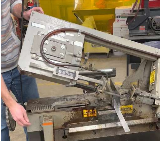
Figure 24: The horizontal saw being utilized to cut the aluminum bar for the clamping mechanism
