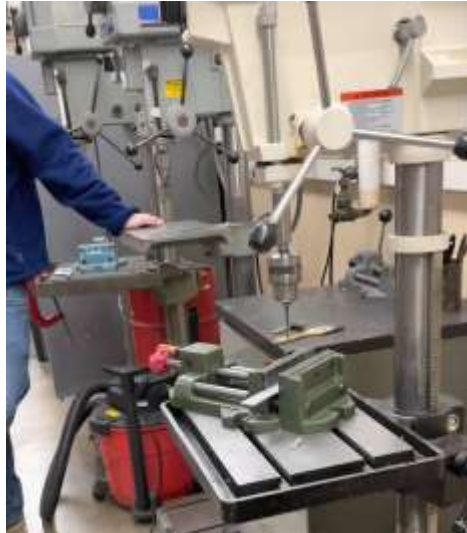
Figure 25: The drill press being utilized to drill out the holes to connect the T-bolt screws to the gantry frame
