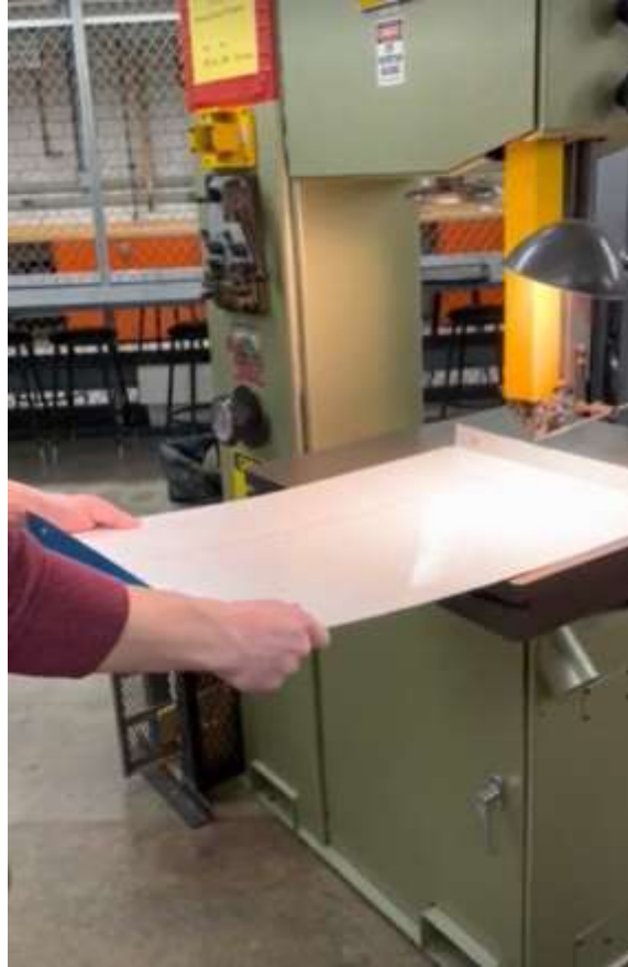
Figure 26: The band saw being utilized to cut the aluminum shield
