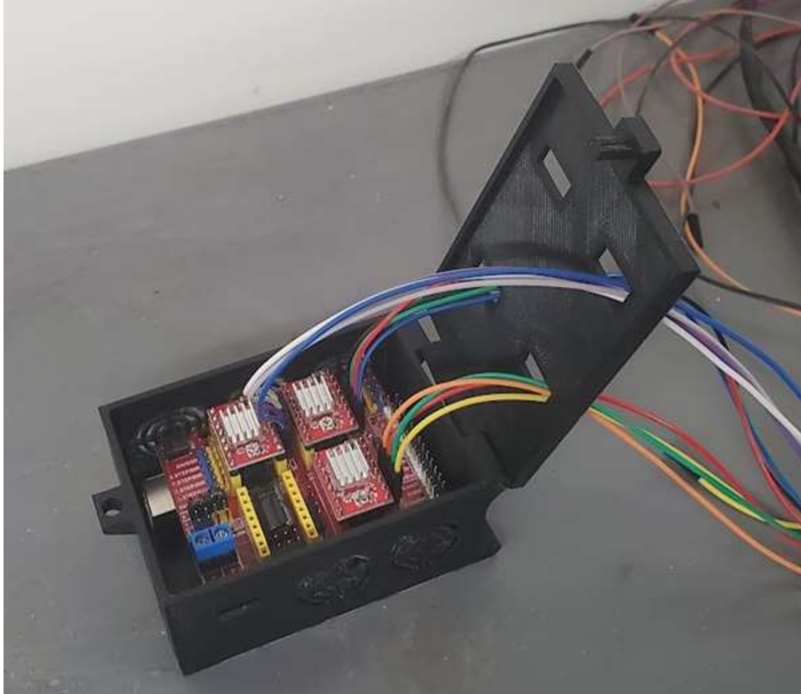
Figure 28: Arduino UNO, CNC Shield, and stepper motor drivers attached to stepper motors
