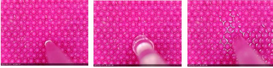
**Figure 5** The relationship between n-octane and the untreated surface in the hexagonal arrangement (250  $\mu\text{m}$  spacing). The droplet failed to retain form on top of the feature and immediately penetrated into the grooves.
