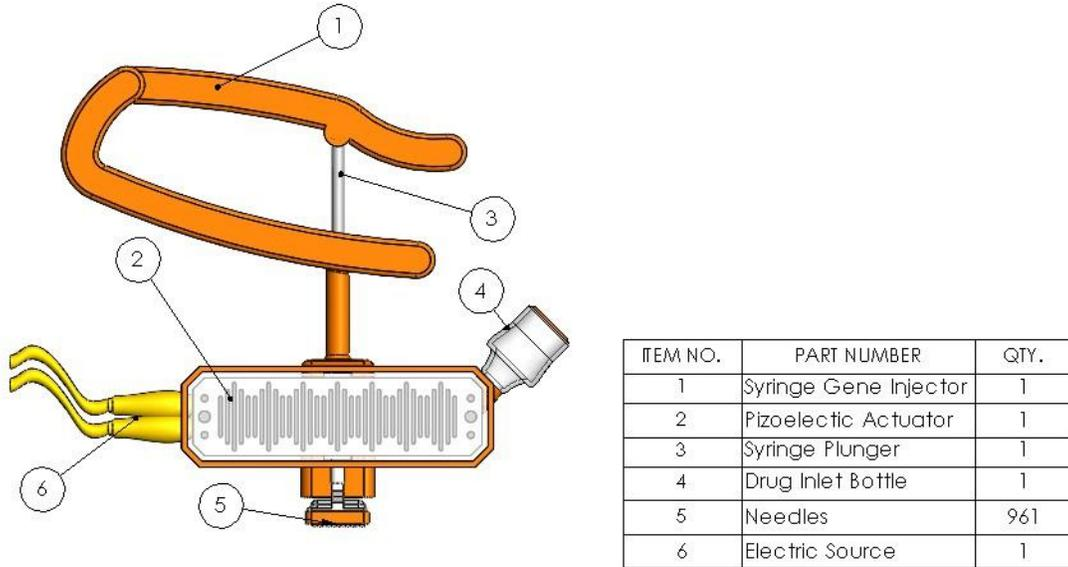
**Figure 4, Parts of device & quantities**
