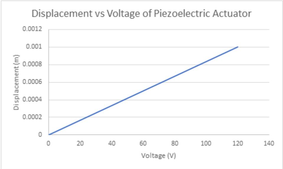
Figure (1) Displacement vs Voltage of Piezoelectric Actuator
