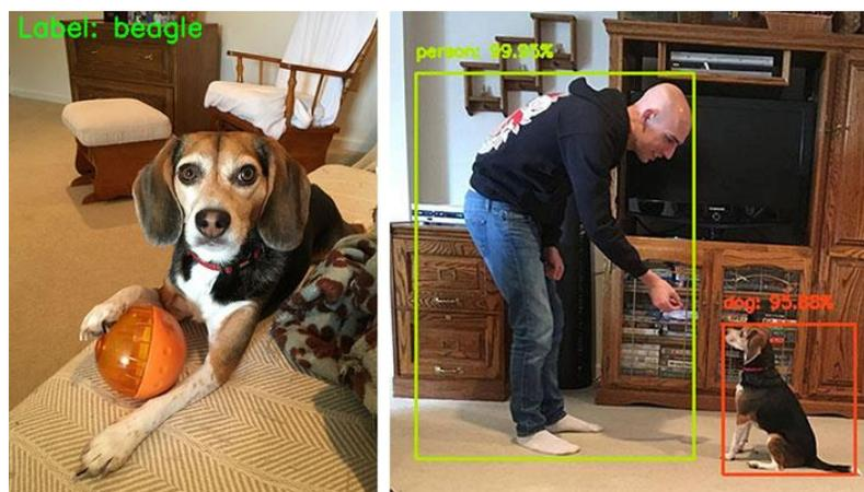
Figure 5: Difference between an image classifier (left) and an object detector (right)
