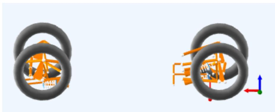
**Figure 13:** ZR19's kinematic pitch center in its center position; this can be assumed to be the pitch center during a steady state driving scenario.
