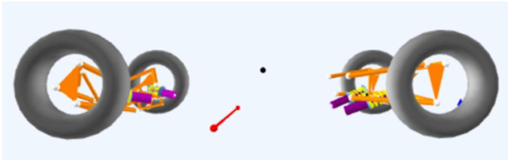
**Figure 17:** ZR20's kinematic pitch center in its frontward-most position during a typical heavy braking scenario.
