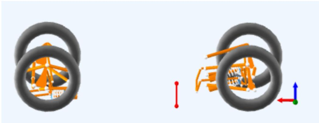
**Figure 14:** ZR19's kinematic pitch center in its forward-most position during a typical heavy braking scenario.
