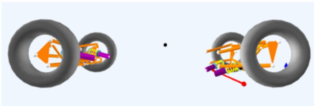
**Figure 15:** ZR20's kinematic pitch center in its most rearward position during a typical acceleration.
