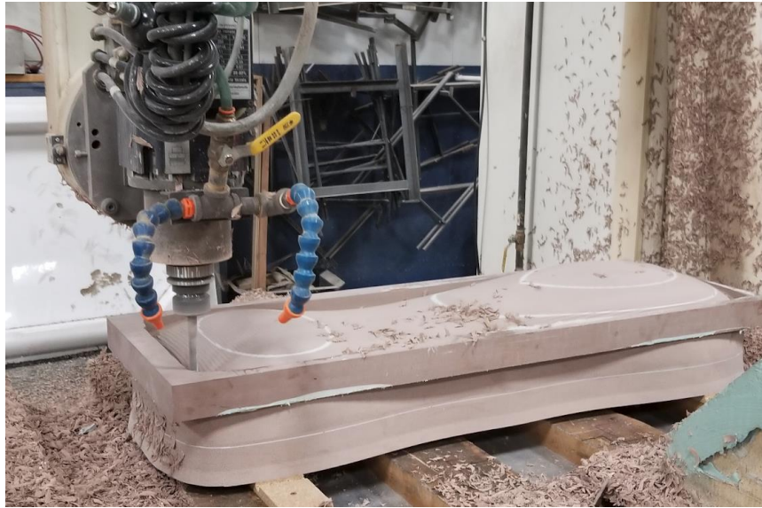
Figure 31: 5 Axis CNC Cutting Tooling
