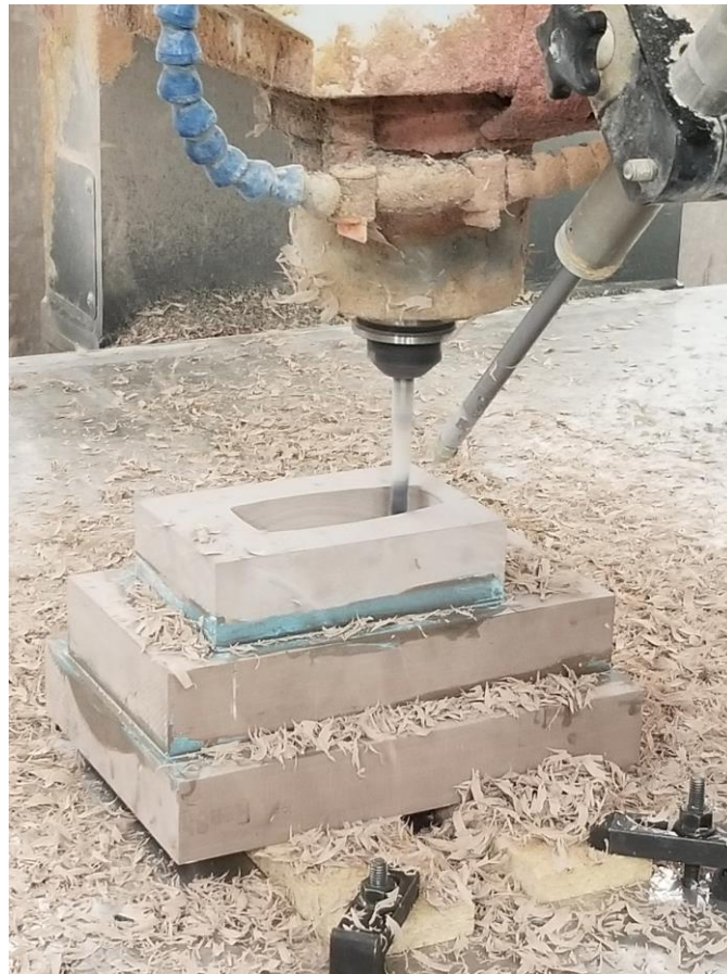
Figure 32: 3 Axis CNC Cutting Tooling
