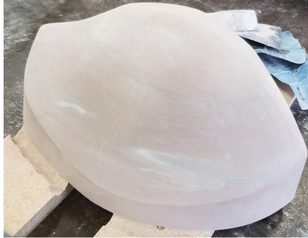
Figure 17: Unfinished Tooling for Pauldron
