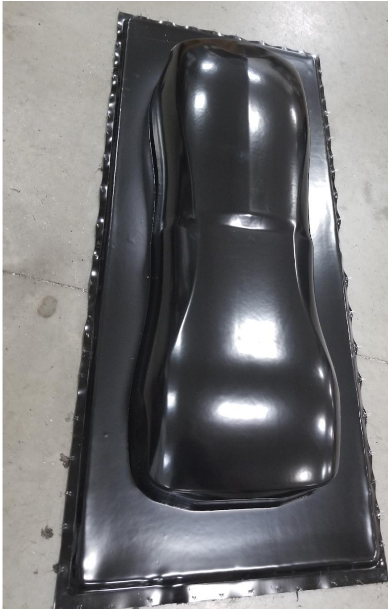
Figure 20: Final Formed Back Piece and Plackart
