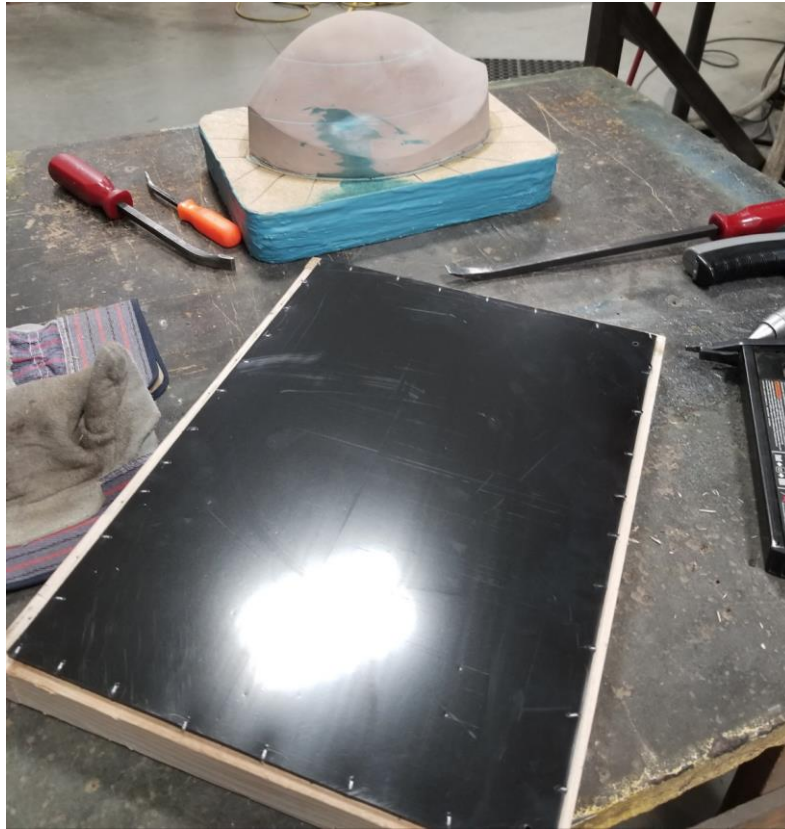
Figure 19: Preparation to Form Pauldrons with Completed Vacuum Box
