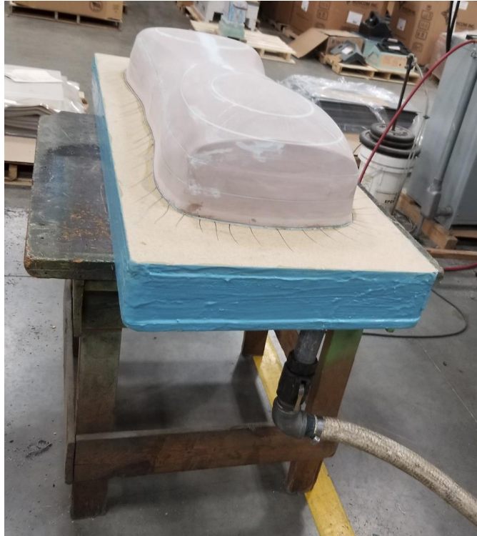
Figure 18: Completed Vacuum Box for Back Piece and Plackart
