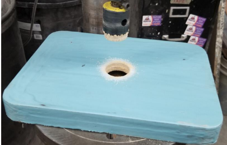
Figure 33: Drilling Hole in Vacuum Box
