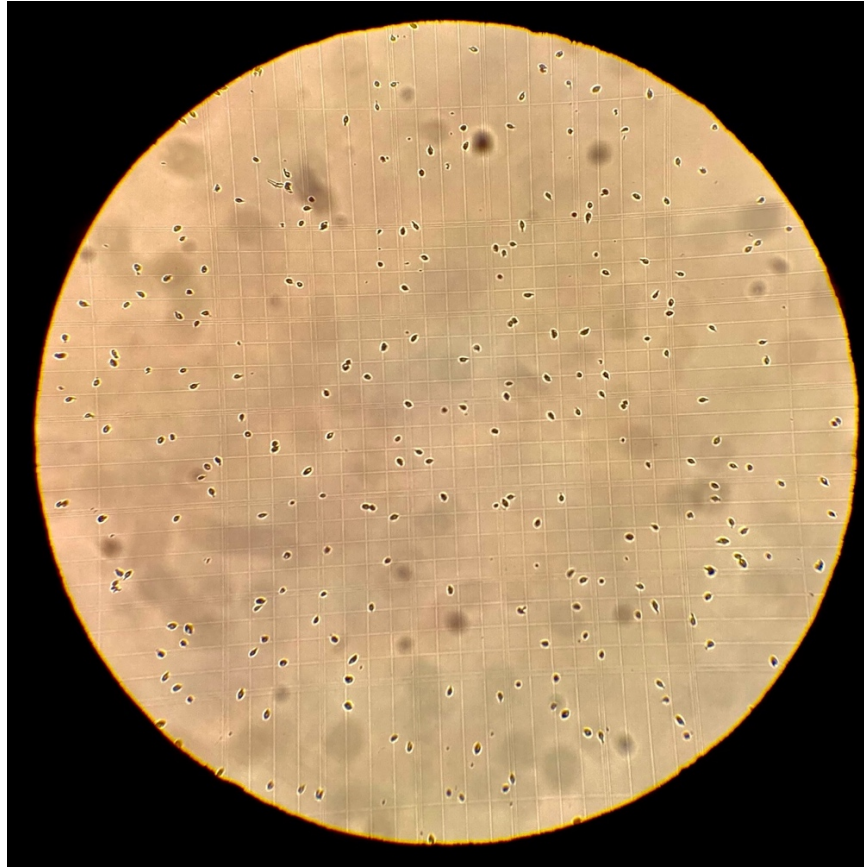
Figure 4 shows the microscopic view of algae cells being counted using a counting chamber. There were microscopic lines carved into the piece of glass placed on top of the chamber. The area of this grid was 1 \text{ mm}^2 and was made-up of a 5 \times 5 square grid and each square contained 16 smaller squares.
