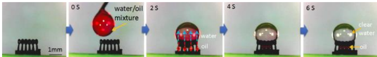
Figure 3. The time scale showing the separation of a water/oil mixture on the 3-D printed eggbeater features studied by Yang et al. Spacing between stalks was varied between 300-500 \mu\text{m} . The height of the stalks was 1000 \mu\text{m} and the diameter of the widest section was 300 \mu\text{m} [1].
