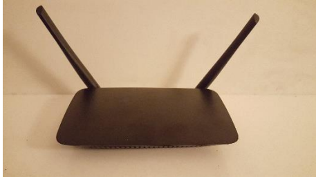
Router A Brand: Linksys Model: N600 WiFi Router E2500 # of Ports: 4 LAN & 1 WAN
