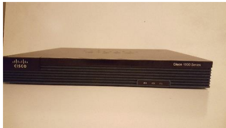
Router C Brand: Cisco Model: Series 1921 # of Ports: 2 Ethernet Ports
