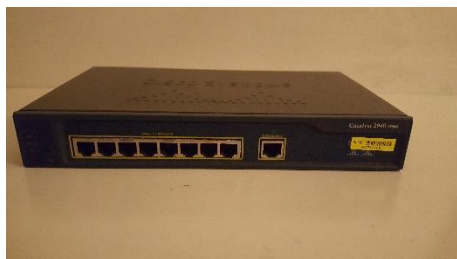
Switch 1 Brand: Cisco Model: 2940 Series # of Ports: 8
