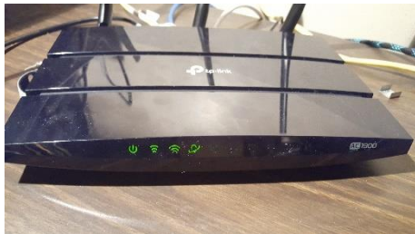
Router B Brand: TP-Link Model: AC1900v6 # of Ports: 4 LAN & 1 WAN
