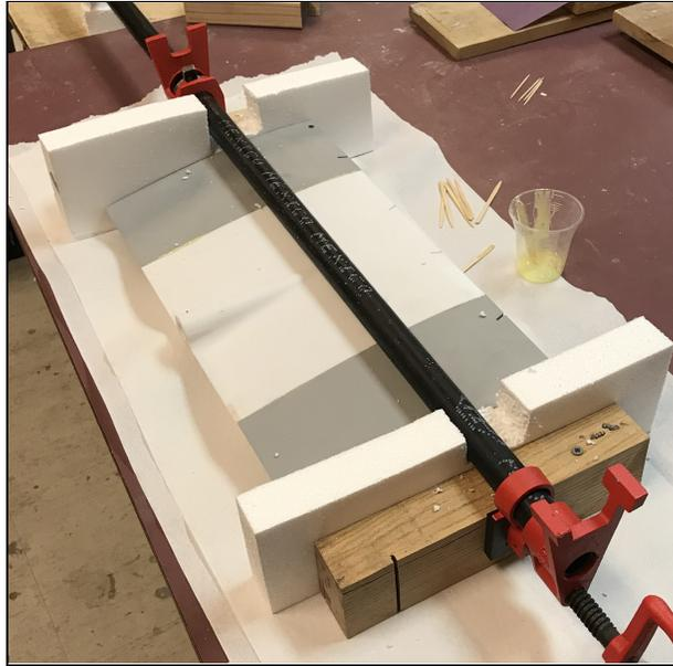
Figure 16 The rear sections being glued together with the clamp, wood, and styrofoam
