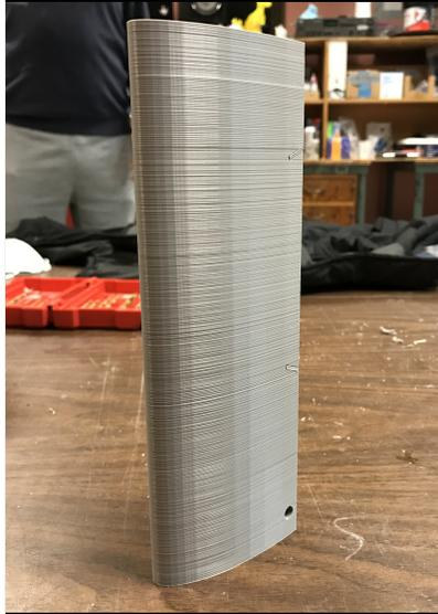
Figure 14 Unsanded leading edge section
