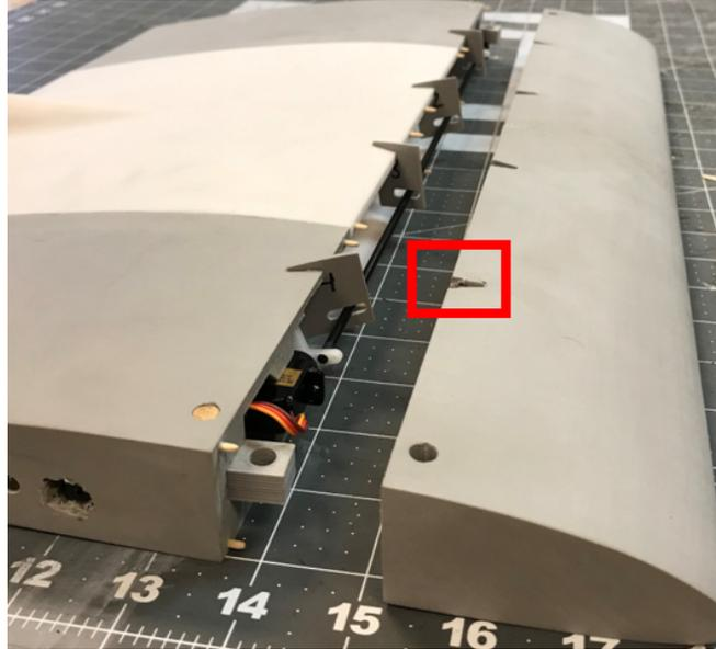
Figure 17 The cut in the leading edge that allowed it to fit around the vortex generators
