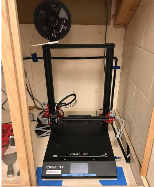
**Figure 13** Zips Aero Design Team CR10s Pro V2 Desktop 3D Printer
