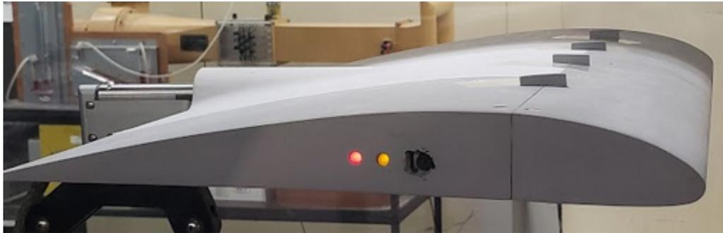
Figure 9 System being tested with button and LED. Light code indicating 40% deployment
