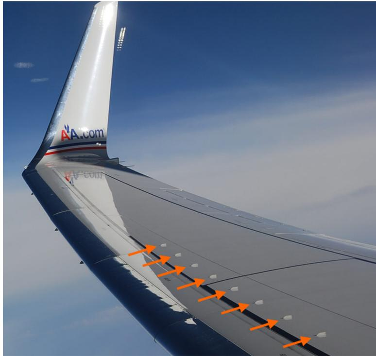
Figure 2 Vortex Generators on the wing of a 737-800 [11]
