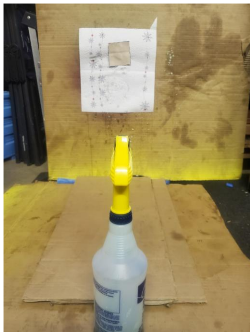
Figure 6. Experimental setup for the droplet adherence testing. A kitchen scale was also used to track how much water was sprayed at each fabric sample.
