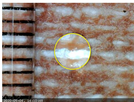
Figure 5. Representation of Image J analysis for a single droplet. The ruler was included in each image to scale the measurements properly. Each droplet was outlined (shown in yellow) using the ellipse tool and the software computed the area of the drawn ellipse.
