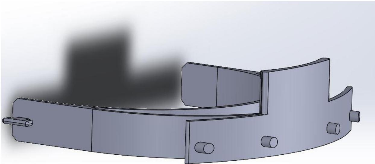
**Figure 7d** Clip on light attachment site
