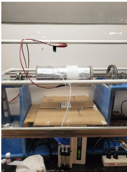
Figure 1: The roller type electrospinning setup used.
