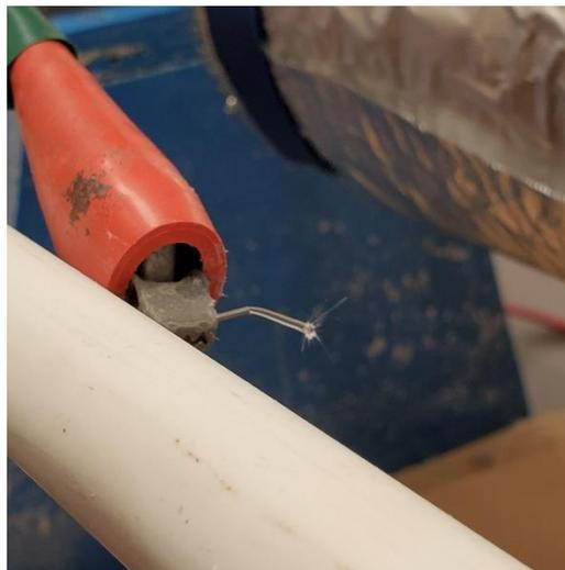
Figure 3: 25 wt% PVDF accumulation at needle tip.
