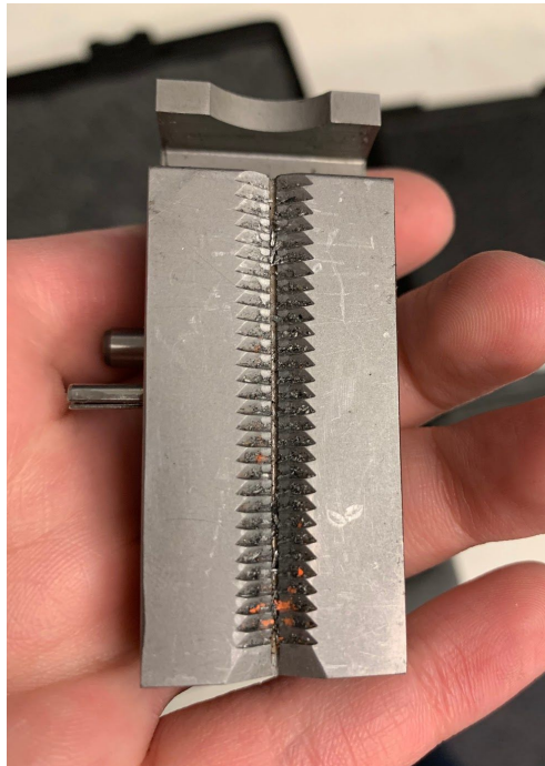
Figure 20: Wedge Grip with Grooved V-Slot from MTS
