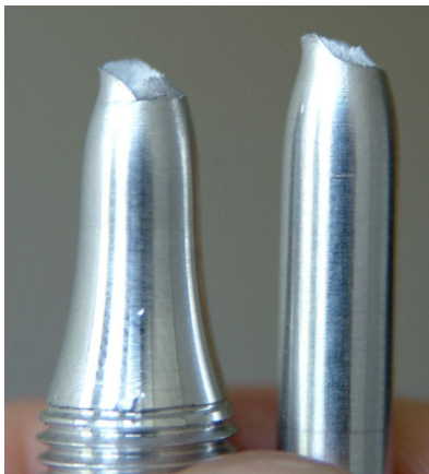
Figure 19: Cup Cone Fracture of Ductile Materials [Ductility]
