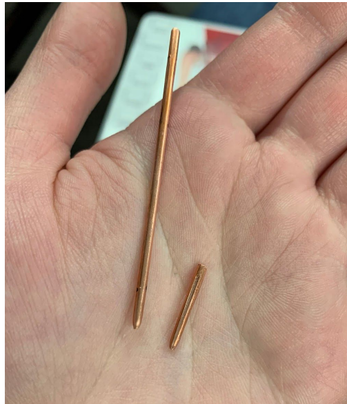
Figure 18: First Break of Copper Wire on Tensile Tester
