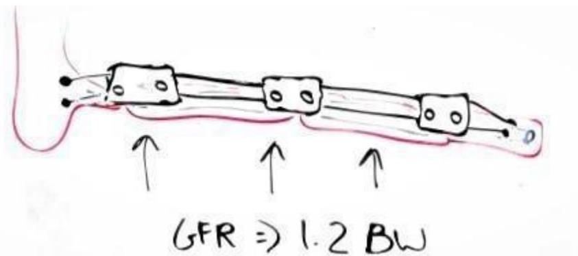
**Figure 5:** Illustration of the load experienced on the Implant System ( $1.2 * \text{Body Weight}$ )
