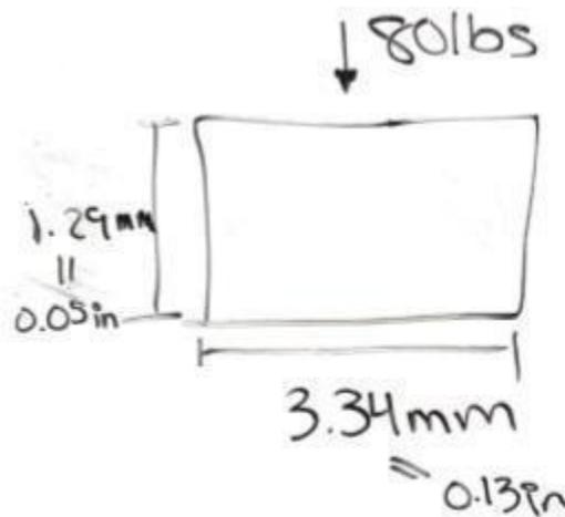
**Figure 6:** Cross-Sectional Area of the T-Plate with Dimensions
