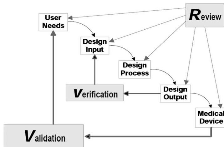
*Figure 1: FDA Waterfall Diagram of Design Controls for Medical Devices [10]*
