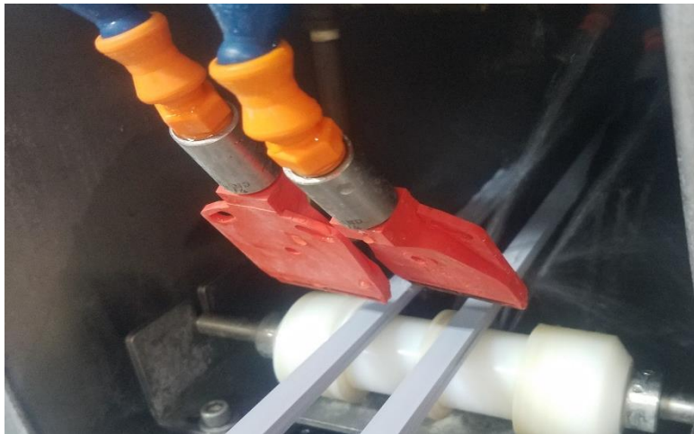
Figure 12: Blower nozzles utilized to limit the amount of hot rinse solution that is carried from the hot rinse tank
