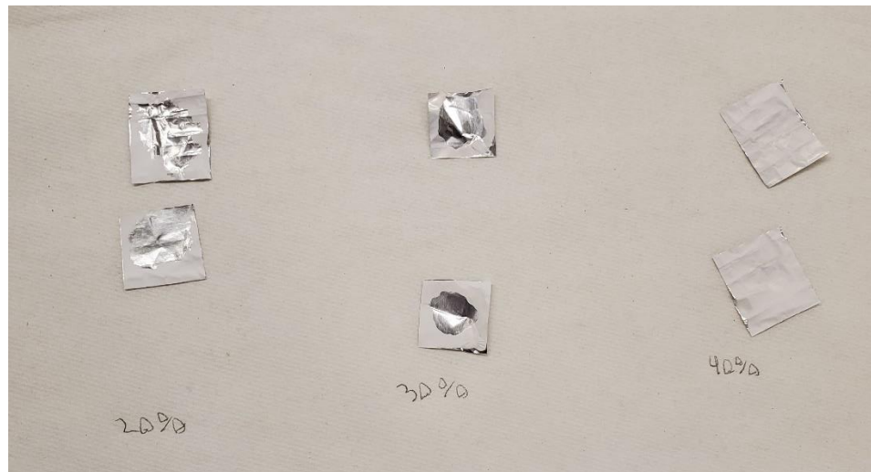
Figure 4: Results of dripping 2 drops of 20, 30, 40 wt% ethanol mixed with acetone on the 10 wt% PVDF fibers
