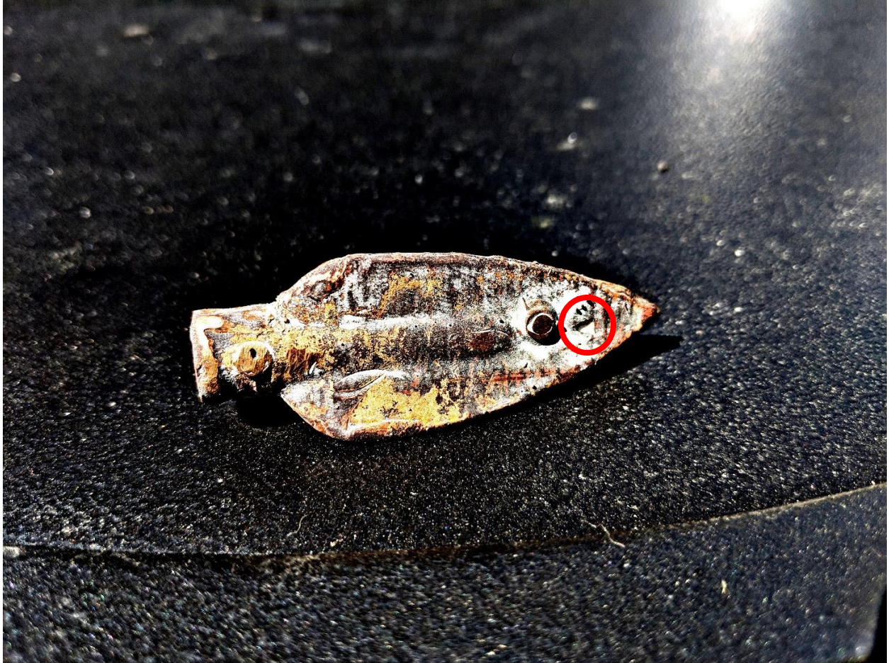
Figure 10. Larger photo of an unpolished trilobate point after casting with another red circle to indicate the small voids left by the casting process. Also visible in this image are the sprues from the casting process. (Image has been adjusted for clarity.)
