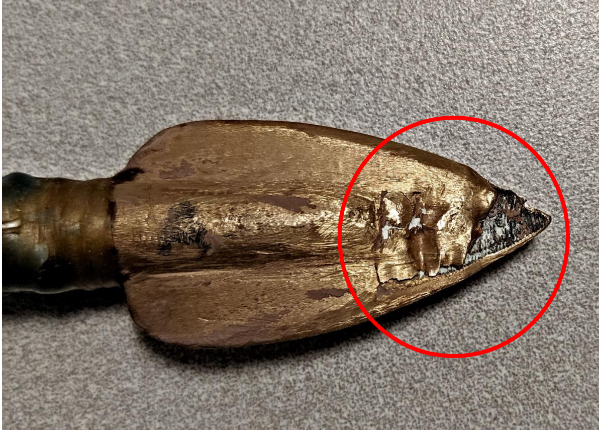
Figure 11. Photo of the bilobate point after being damaged from a misfire and repaired through cold-hammering. The image also shows the extent of the void in the point. While the size of the void was clearly larger than the other arrowheads initially, the full extent of it was not apparent until after it was damaged. (Image has been adjusted for clarity.)
