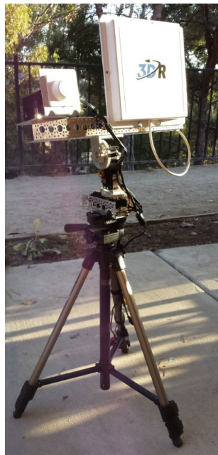
Figure 4b: Command Station Antenna Array
