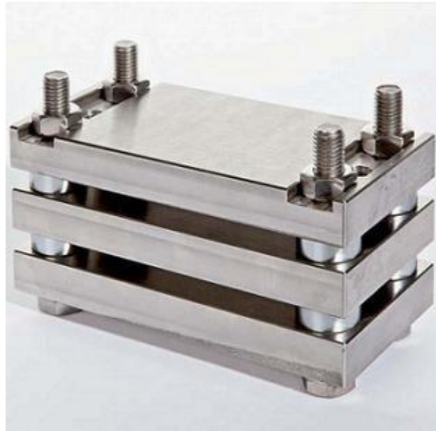
Figure 2. A picture of a compression set device with a similar design to the ones that were used in this project. The spacers, compression plates, nuts, and bolts that make up the device are easily visible.
