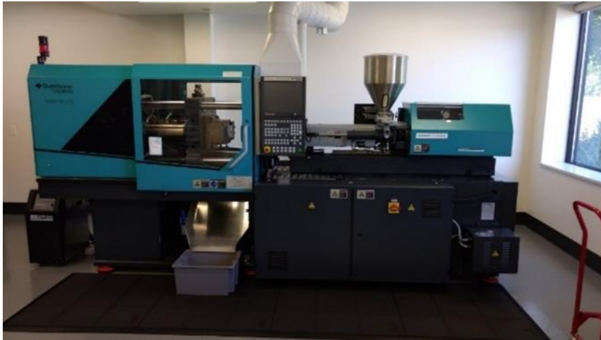
Figure 13. The above figure is a picture of the Injection Molding Machine that was used to make TPV compression set button samples that were used for compression set testing.
