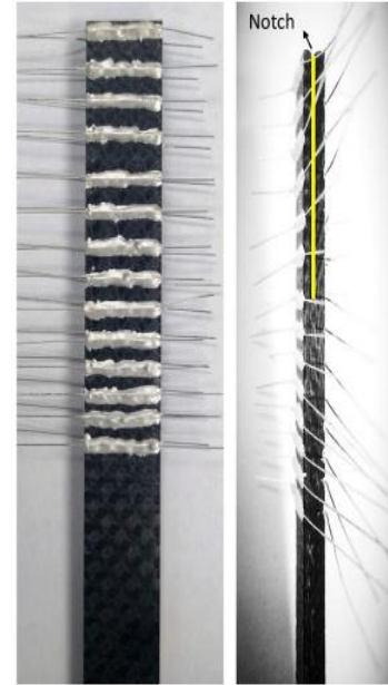
Figure 2: Electrical leads attached to tensile tested specimen 2
