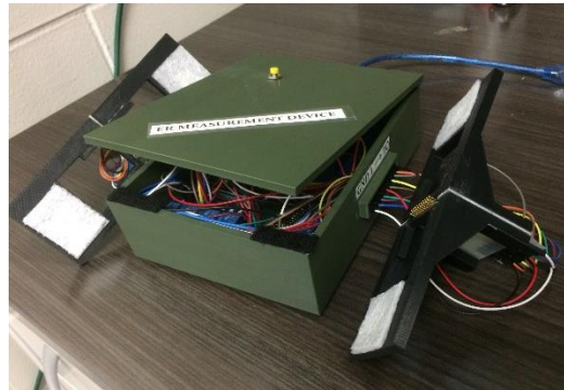
Figure 10 (b): 3D printed probe fixture and DAQ box
