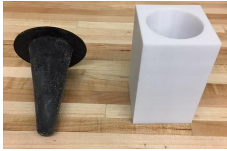
Figure 19. Completed two-piece mold.
