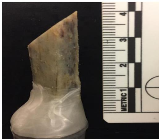
**Figure 9.** An image of a left sixth rib sample secured to a brass mount with dental wax and Parafilm before scanning in the SkyScan 1172 desktop X-ray system. Ruler on the side to indicate average sample length.
