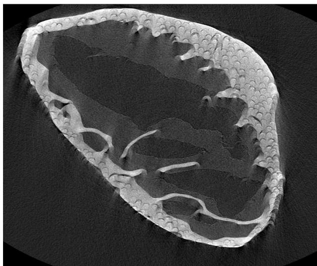
**Figure 11.** A cross-section of a rib sample in NRecon prior to manual adjustment. The cortical pores are nearly impossible to differentiate.
