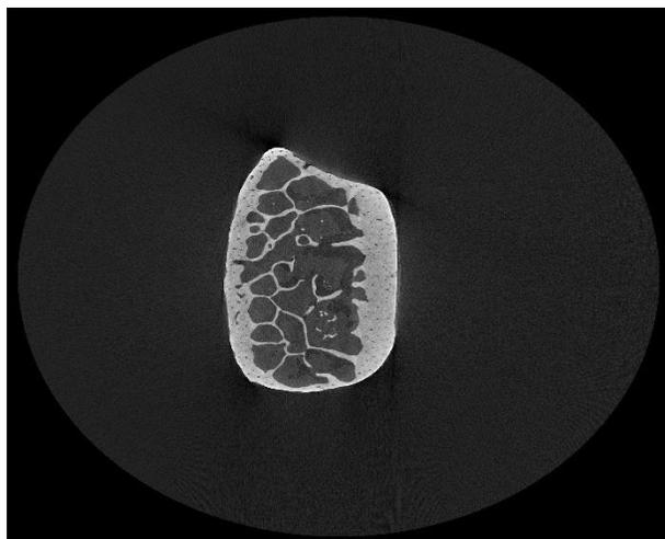
**Figure 13.** A cross-section of a rib sample in NRecon prior to quantitative analysis with CTAnalyser. Without a Region of Interest (ROI) specified, the program would try to take measurements on everything within the grey circle.
