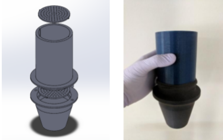
Figure 4: The testing apparatus designed for this study. Left - The model in SolidWorks, Right - The 3D printed fully assembled apparatus.
