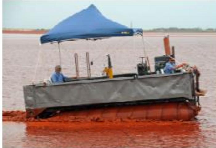
Figure 5: Amphibious vehicle used for creating trenches (Atvhire).
