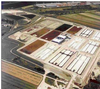
Figure 4: Lagoon dewatering facility (Foged, S., et al.).
