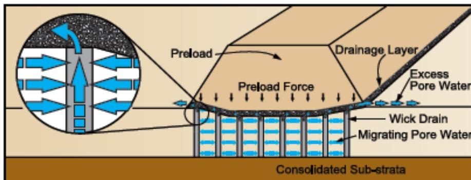
Figure 8: Cross section of PVD system ("Wick Drains" 2013).
