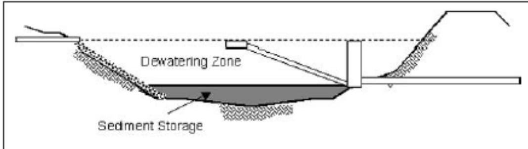
Figure 1: Settling basin dewatering zone and sediment storage (Mathews & Mecklenburg 2006).
