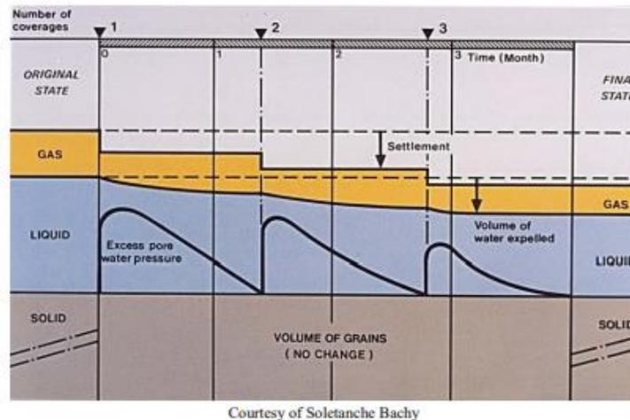
Figure 6: Phase diagram during dynamic compaction (Schaefer, et al. 2016).
