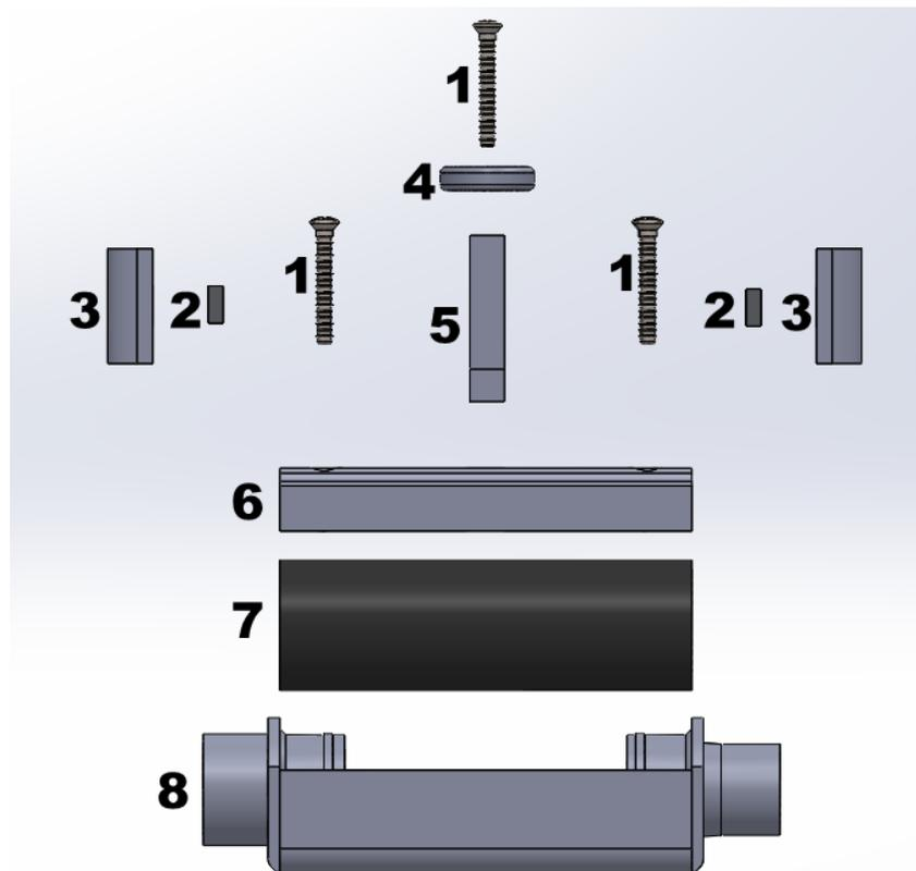
*Figure 3.* Exploded view of the device. 1 - Self-tapping screws. 2 - Neodymium magnets with adhesive. 3- Safety cage. 4 - Top cap for plunger. 5 - Plunger Body. 6 - Upper housing of main body assembly. 7 - Silicone tubing. 8 - Lower housing of main body assembly.
