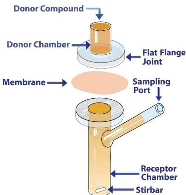
Figure 1: Setup of a Franz Cell
