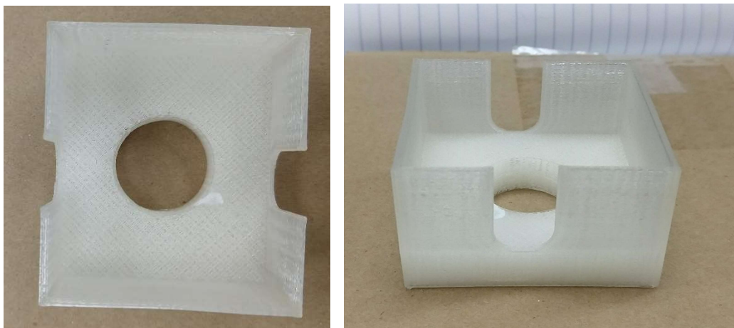
Figure 3A and 3B: Top and side view of membrane testing prototype
