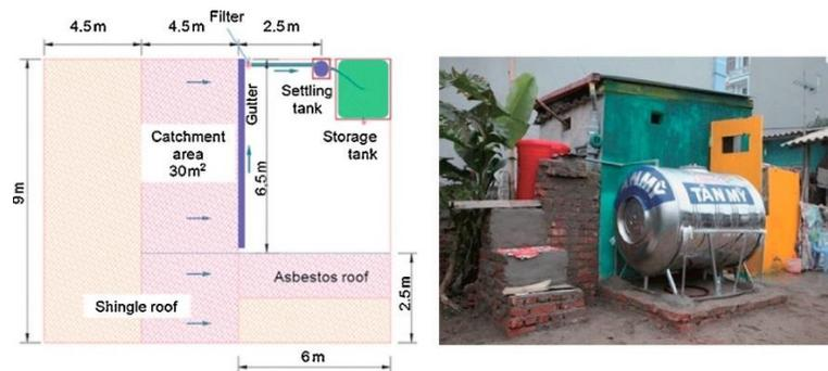
Figure 6 – Rainwater harvesting tank in Hanoi [10]
