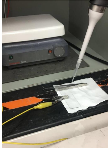
Figure 1: Pictured on top is the setup used for analyzing each sensor by attaching it the electrodes and dropping solutions of varying sodium ion concentration.
