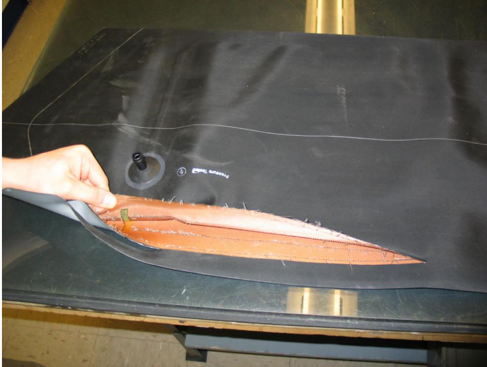
Figure 11 shows Deicer A Burst test bondside failure
