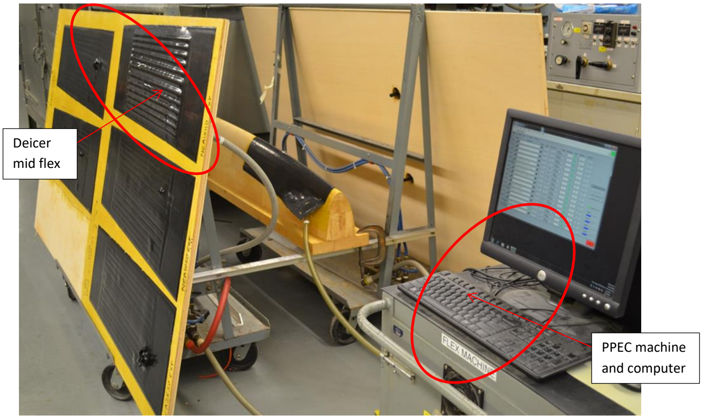
Figure 10 shows the PPEC flex machine. The computer controls the settings for each channel. The deicers are mounted to boards and the top right one is shown mid flex.
