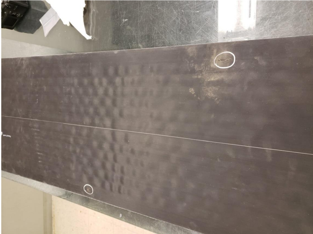
Figure 14 shows Exp Deicer A Burst Bondside failure
