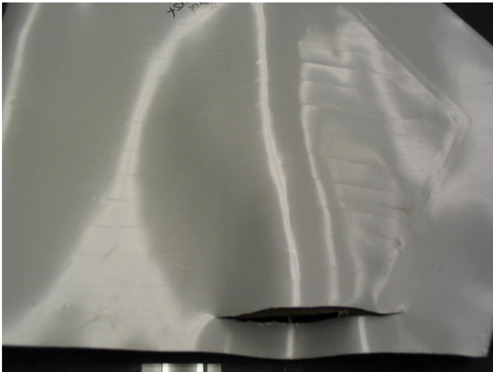
Figure 12 shows Deicer A Burst test breezeside failure
