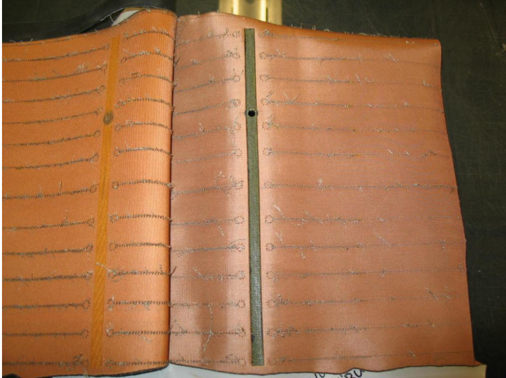
Figure 13 shows Deicer A Burst test manifold inspection
