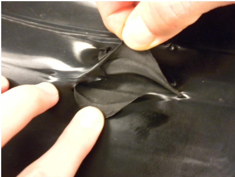
Figure 17 shows Exp B Deicer B 2 cross-inflation inspection.
