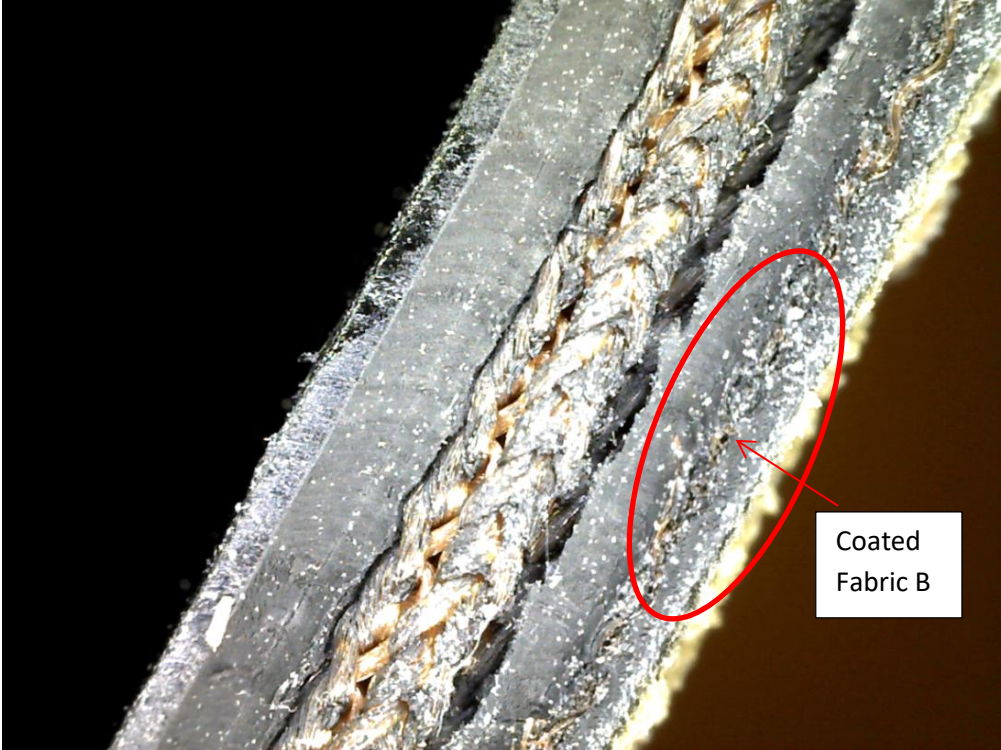
Figure 18 shows Deicer B 1 cross-section. As shown, there is no delamination in the layer containing Coated Fabric B.
